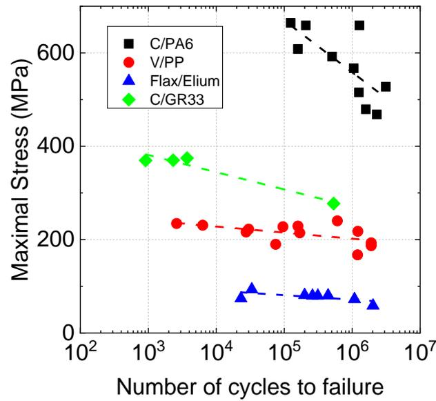
Figure 11: Flexural fatigue strength of alternative materials
