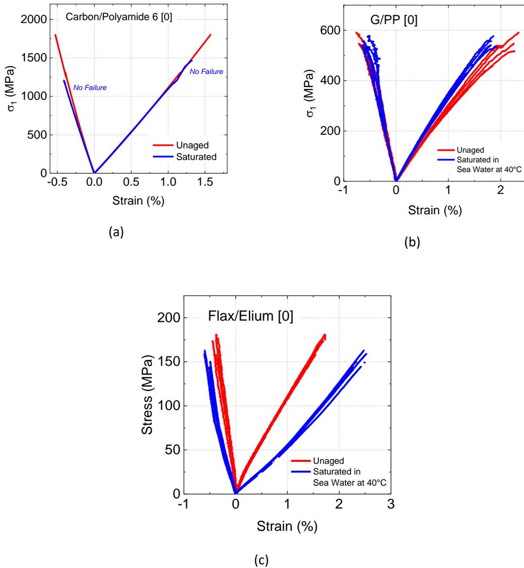
Figure 20: Effect of sea water aging on the longitudinal properties of (a) Carbon/Polyamide 6 (b) Glass/Polypropylene (c) Flax/Elium
