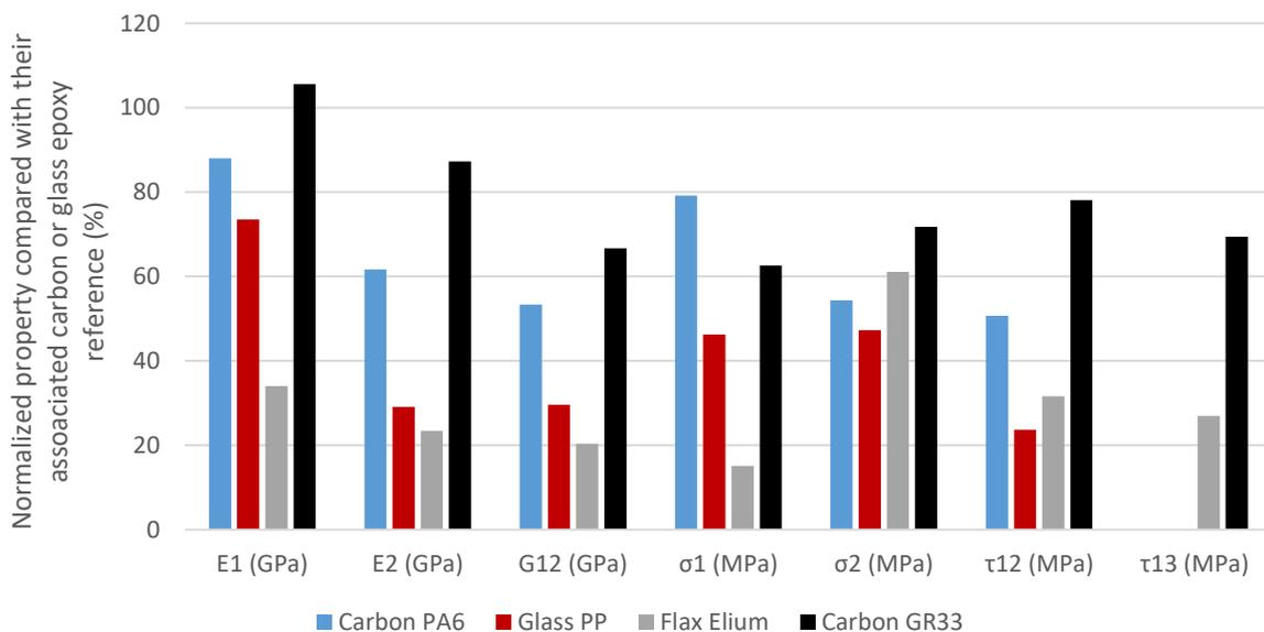
**Figure 14: Properties of alternative materials normalized with respect to their carbon and glass epoxy references from T1.3**
