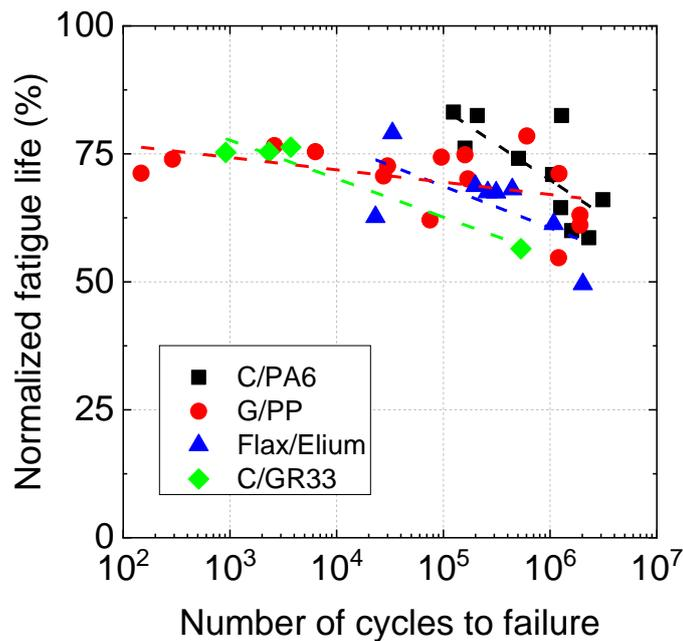
Figure 12: Flexural fatigue results normalized by flexural static strength
