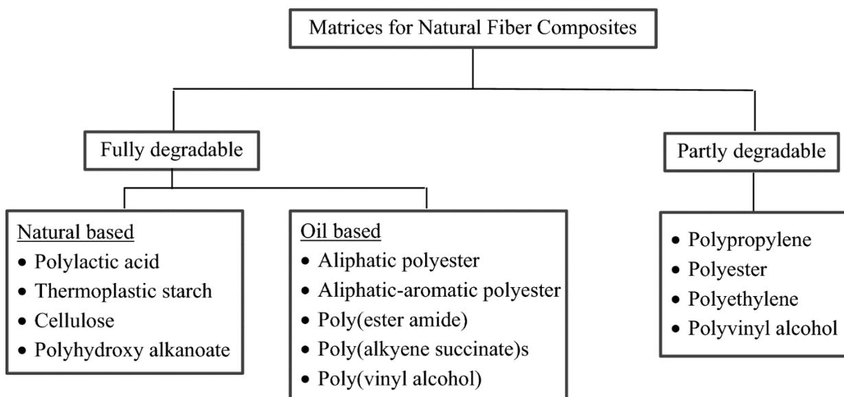
Figure 2: Classification of polymer matrices for natural fibre composites [1]
