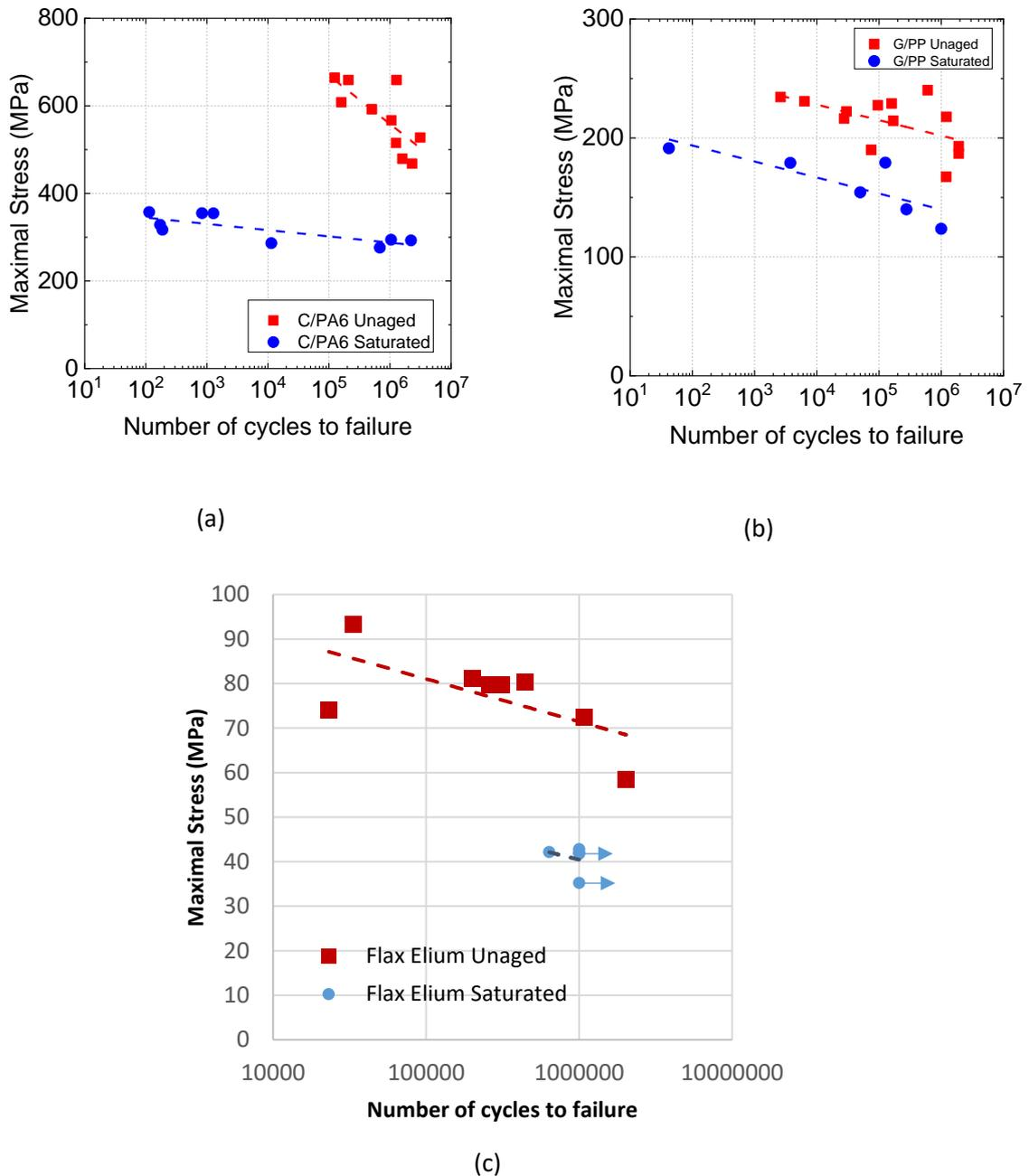
Figure 13: Effect of sea water aging on the flexural fatigue properties of (a) Carbon/Polyamide 6 (b) Glass/Polypropylene (c) Flax/Elium
