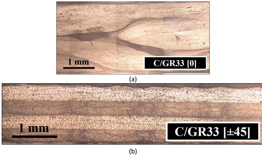
Figure 8: Polished sections for specimens extracted from the C/GR33 panels (a) [0] (b) [±45]
