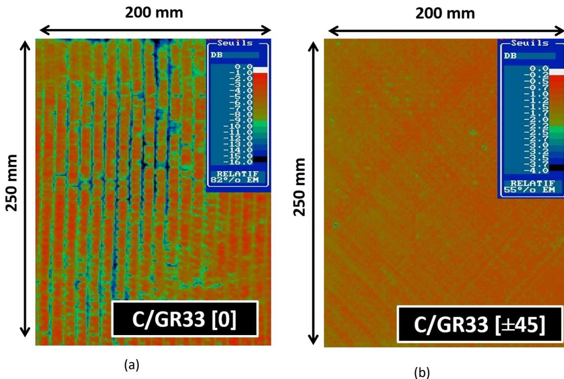
Figure 6: Ultrasonic C-scans on the Carbon/GreenPoxy 33 panels (a) [0] Attenuation scale = 16 dB (b) [±45] Attenuation scale = 4 dB
