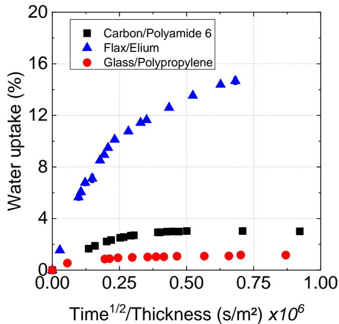
Figure 10: Sea water absorption during immersion at 40°C
