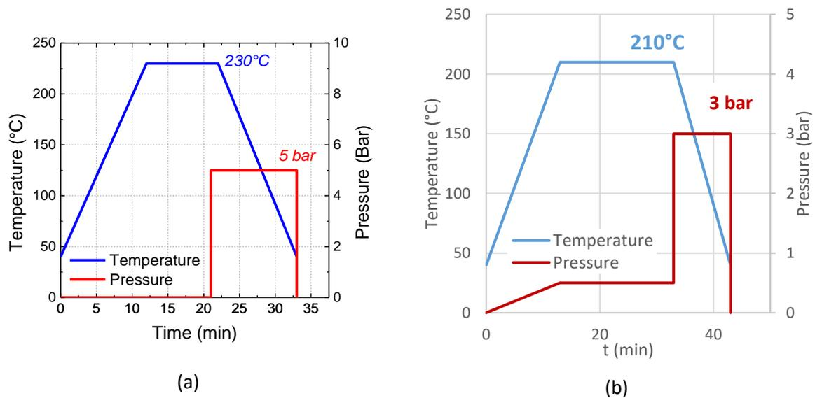
**Figure 4: Manufacturing cycles for thermoplastic composites (a) Carbon/Polyamide 6 (b) Glass/Polypropylene**
