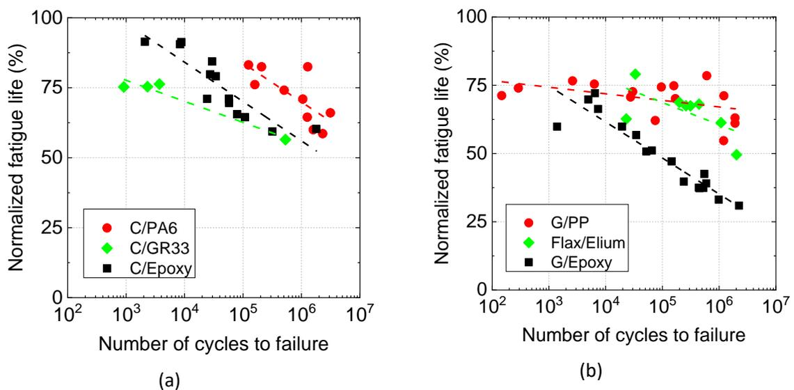
**Figure 15: Normalized fatigue strength by static test values in the unaged state (a) Carbon based materials (b) Glass based materials and F/EI material**
